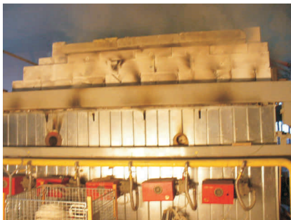
Picture of chamber for fire testing acc. to DIN 4102-12
